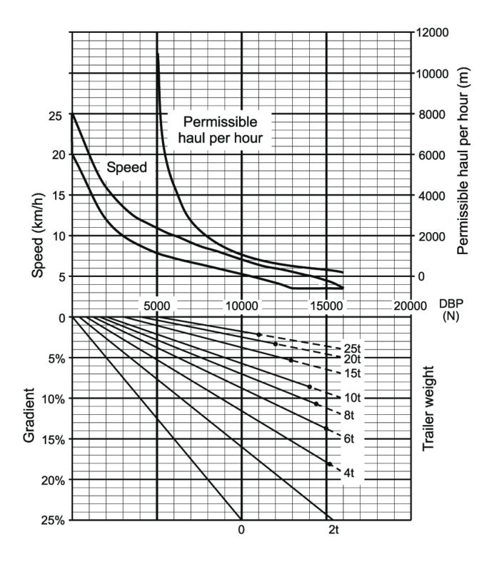
Load/gradient combinations shown by full line can be restarted from stationart on the gradient..
