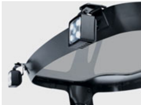
LED working spotlights: bright, modern LED technology for optimum visibility
