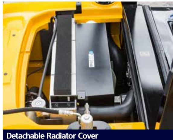
The plastic toolless radiator sub hood on top of the counterweight, separated from the main hood, allows for greater access and reduces the downtime for checking the coolant level and servicing the radiator.
