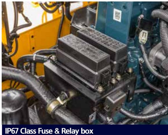
The fuse and relay blocks, which are vulnerable to contamination, are contained in a water and dust tight box that is installed in the engine compartment for ease of access when maintenance is required.
