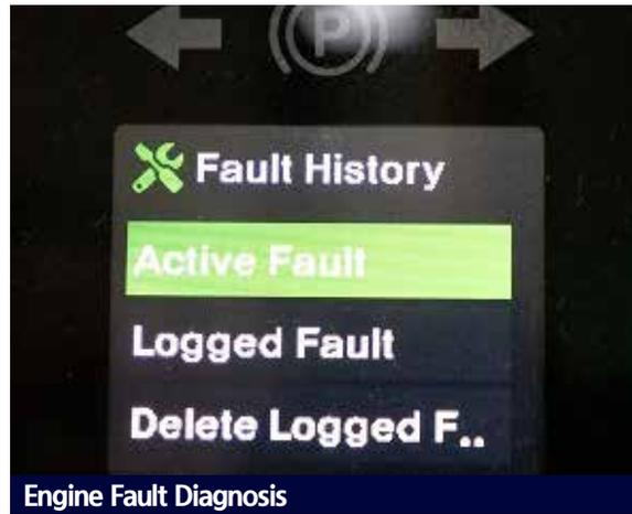
The equipment's fault codes, which are recorded and stored by ECU and MCU, are easily accessible on the cluster screen without any additional tools to ensure rapid and precise diagnostics and repair.
