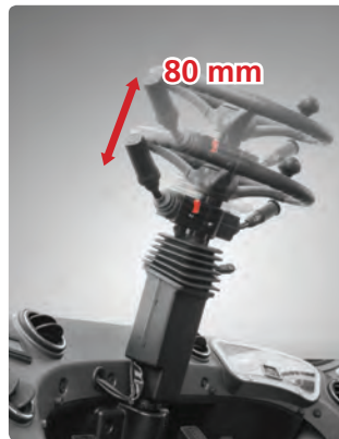
Adjustable Steering Wheel Steering wheel with horn button can be adjusted by a lever on the right-hand side for the most comfortable operator position.
