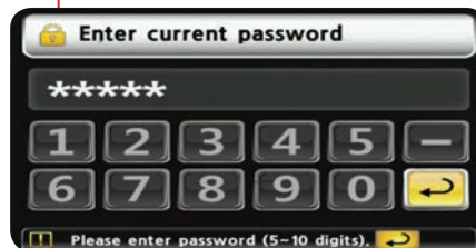
Password-protected starting system (anti-theft system)
