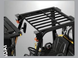
**Strong Overhead Guard** The safety overhead guard meets ISO 6055 regulation and protects the operator during hazardous jobs.
