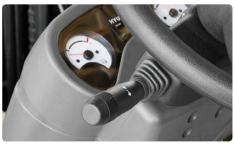
**Easy and Safe Shift Lever** A single lever on the left side of the steering column gives the operator fast, easy control of direction. The lever must be in the neutral position before the engine can be started.
