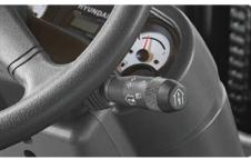
Secondary Horn Secondary Horn gives access to lights and horn
