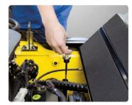
Easy Maintenance Oil Check The T/M oil level can be checked
