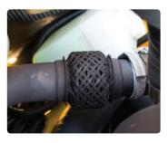
**Expansion Bellows** The expansion bellows absorbs vibration and reduces noise generated from the exhaust system and also extends the life cycle of exhaust system.
