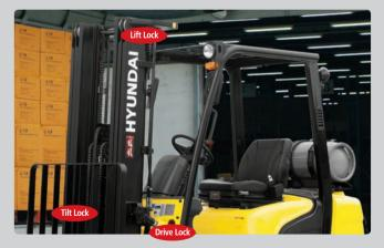
**OPSS (Operator Presence Sensing System)** Control of mast tilting, lifting and lowering is not possible through operation of the appropriate control when the operator is not in the seated position
