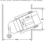
Aisle dimensions listed above assume the minimum bay width to be straddle OD plust 6" (2.5" on either side of straddle leg). Truck performance may vary due to applica-tion requirements and changes in model design.
