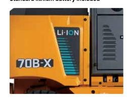
Comes equipped with high-performance lithium batteries for extended run time and fast charging, improving uptime and efficiency.
