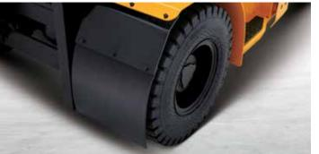
Shields the operator and truck from debris and contaminants kicked up from the front tires.
