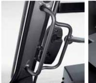
A dedicated mounting bar to the right of the driver's seat and a built-in storage compartment below the cabin help create a personalized and efficient work environment.
