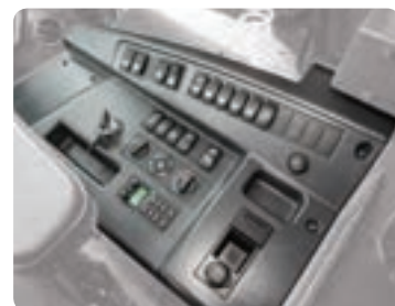
Centralized Instrument Switch Panel
