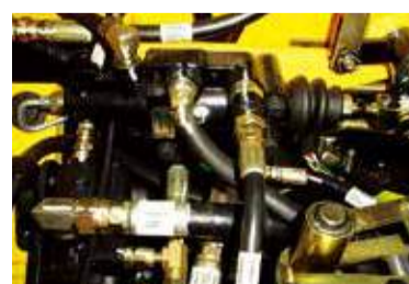
Boosting-Type Brake Valve (OPT)
