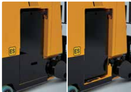
Battery Side Gate Interlock Sensor The system prevents accidents due to an improperly installed battery side gate. The system prevents travel if the battery side gates are not properly installed. This is a standard feature.
