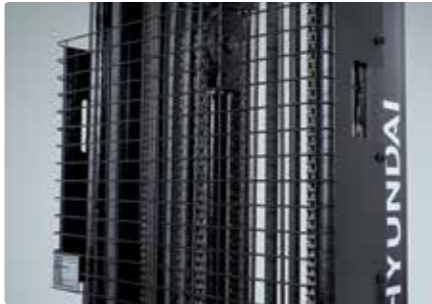
Protection Screen Protection screen installed between mast and operator room for safety.
