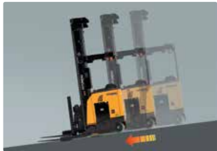
Anti Roll Back For greater safety, this system prevents the forklift from rolling rapidly down a slope when the control handle & brake pedal are not applied while also offering improved ramp start-up abilities.
