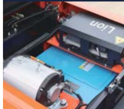
Open design for controller and lifting motor, more convenient maintenance
