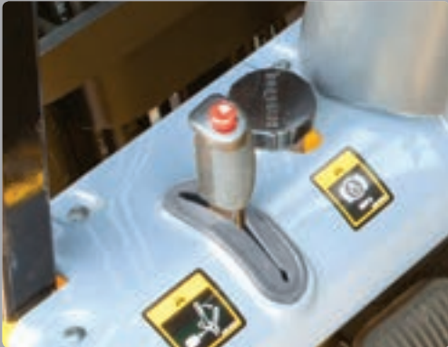
Parking Brake Ratchet type parking brake is durable and easy for the operator to set.
