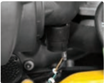
Electrically Monitored Air Filter Air cleaner sensor alerts the operator of a restricted air filter and allows replacement before damage.
