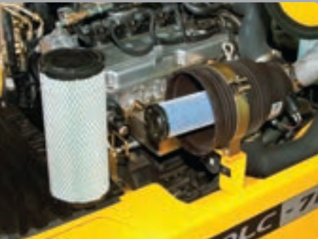
Easy Change Air Cleaner The air filter is readily accessible for cleaning or replacement. (6inch Cyclone Type)
