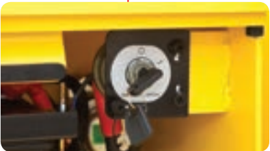
Master Switch A master switch disconnects the battery power to protect the electrical system from excess electrical drainage.
