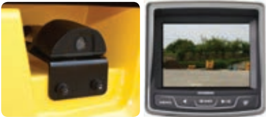
Rear View Camera The rear view camera provides great rear visibility, and the monitor supports 4 camera channels for operator convenience.
