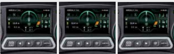
N (Normal) : Same acceleration feel as ICE forklifts H (High) : Provides instant acceleration performance for fast task processing E (Economic) : Smooth acceleration performance with energy efficiency
