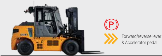
Auto hold: Automatically engages the parking brake when the brake pedal is held for more than 4 seconds. Auto parking: Automatically engages the parking brake when the operator leaves the seat.
