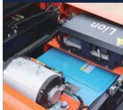
Open design for controller and lifting motor, more convenient maintenance
