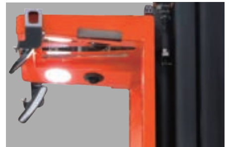
LED work lights and fan
